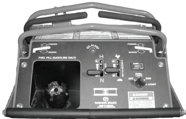
This photo shows the hydrostatic control levers are in the neutral position.
