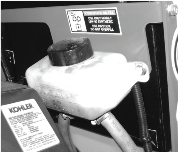
Hydraulic Oil expansion tank and filler (Fill to bottom line when cold.)
