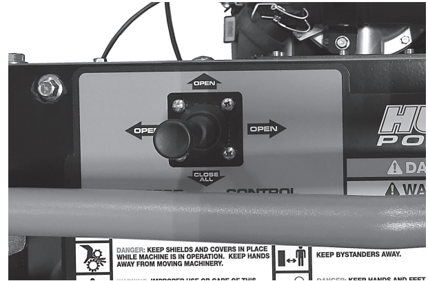
Deflector Control Switches
